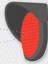
LED SYSTEM multiple LED packages + supporting electrical, thermal, optical, and mechanical components
